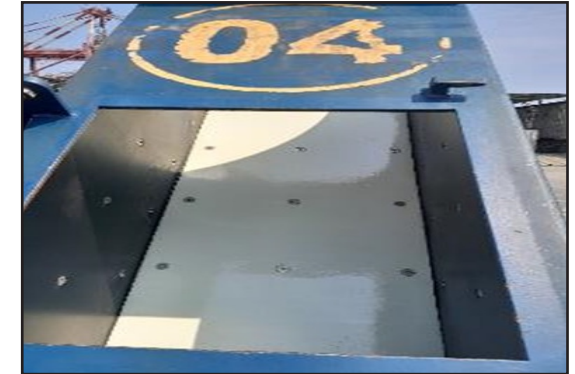
ARC MX FG coating has extended the chute life from 8 months to over 3 years.
